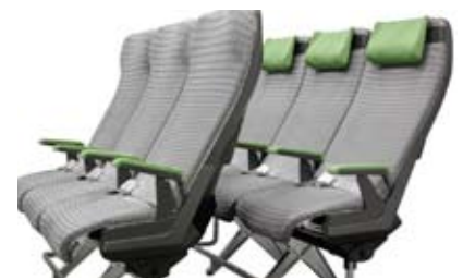
Aircraft seats with cantilever knitted structure (Photo: Kobleder Strickmoden)
